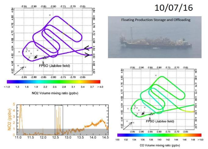
**Figure 6:** NO2 and CO mixing ratio in ppbv measured on board the DLR Falcon 20 on 10 July 2016. High values of NO2 were observed in a narrow plume of a FPSO vessel in the Gulf of Guinea, off the coast of Ghana (From V. Brocchi, V. Catoire – Univ of Orleans, H. Schlager - DLR)
