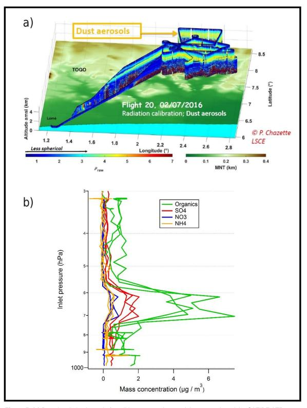
**Figure 5**: (a) Raw depolarization ratio from lidar measured on 02 July 2016 on board the SAFIRE ATR42 aircraft. Dust layer are well identified in the northern part of the flight (From C. Flamant, P. Chazette - UPMC). (b) C-ToF AMS observations of sulfate, nitrate and ammonium on board the DLR Falcon on 6 July 2016. High concentrations between 750 and 600 hPa could be due to a biomass burning layer (From A. Batenburg, C. Schulz, J. Schneider, and S. Borrmann – MPI Mainz)
