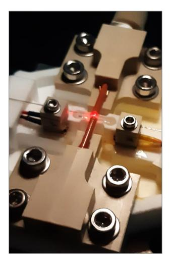
We build fibre microcavities to characterise nanoparticles in aqueous suspensions.
