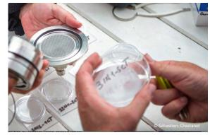
Filters with aerosol impactors
