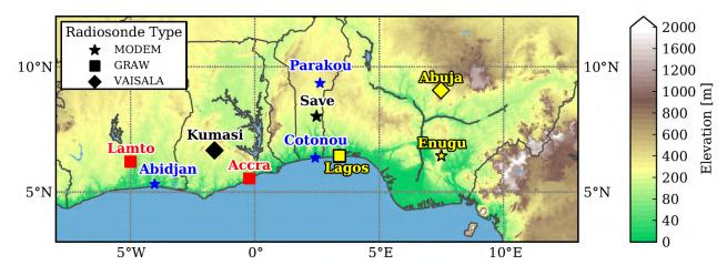
DACCIWA Radiosonde network and deployed sonde types. Blue: Operational or re-activated AMMA stations with enhanced sounding frequency; Black: DACCIWA super-sites; Red: DACCIWA stations operated by KIT, GMet, and UFHB; Yellow: Operational ASECNA and NWS stations outside the DACCIWA network
