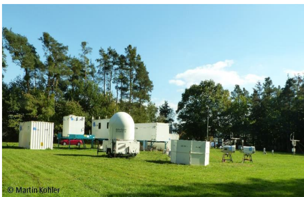
Test setup of KITcube at Karlsruhe in Germany. In the foreground from left to right the x-band rain radar, sodar, microwave radiometers and energy balance station can be seen. In the rear, transport containers, wind lidar and office containers are visible.
