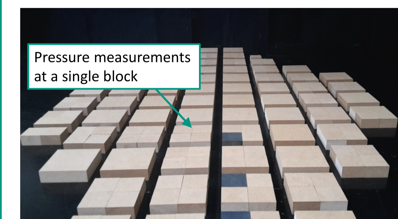
Fig. 6: Photo of the experimental setup. Block array represents an idealized city. Pressure distribution was measured at a single block in the array (scale 1:800).
